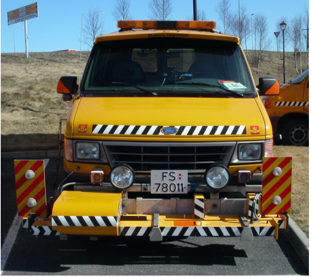
Figure 8: Vehicle "ALFRED" used for measurement of road surface unevenness and texture.
