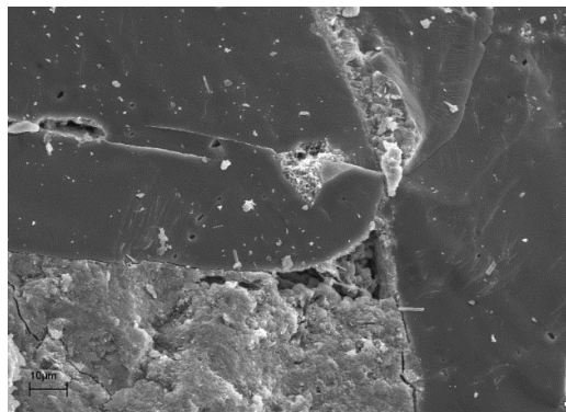
5. Spalling of Portlandite.
