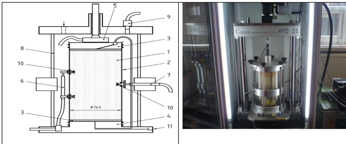
1. Specimen, 2. Membrane, 3. Specimen cap, 4. Specimen base,
