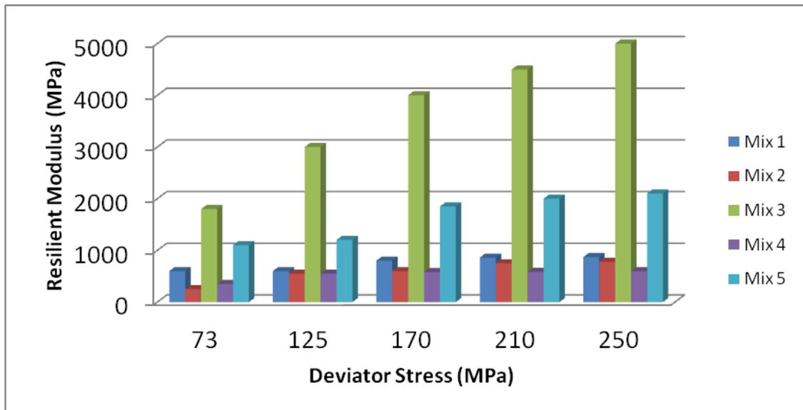
Figure 4. Resilient modulus of control mixes compared with the mixes containing waste dust with and without GBS.
