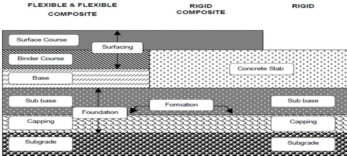
Figure 1. Different Pavements and Their Foundations (Wanab, Y. 2005)
