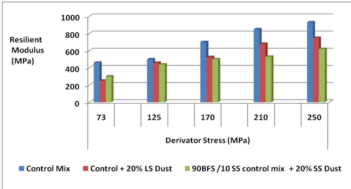
Figure 3. Resilient modulus of control mixes compared with the mixes containing waste dust
