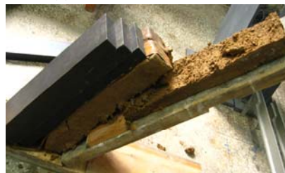
(b) The final broken forms of specimen with freezing and thawing (F-T) interface
