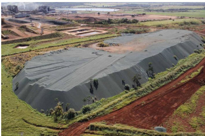
Figure 5 – Slag stocks formed during the first years of operation of Barro Alto.
