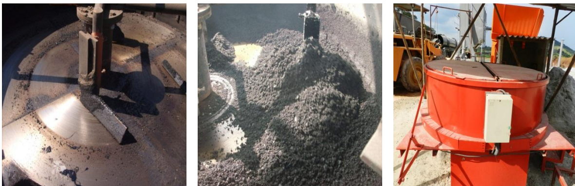
Figure 4. View of the mixing pallets and homogeneous aspect of the mix obtained by the equipment J-1000.
