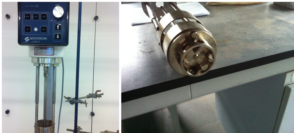
Figure 1: Laboratory high shear mixer used in this study (left), and specially designed head for blending polymer pellets (right)
