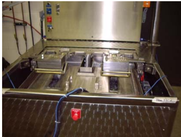
Figure 2: Loaded wheel test setup with air condition chamber
