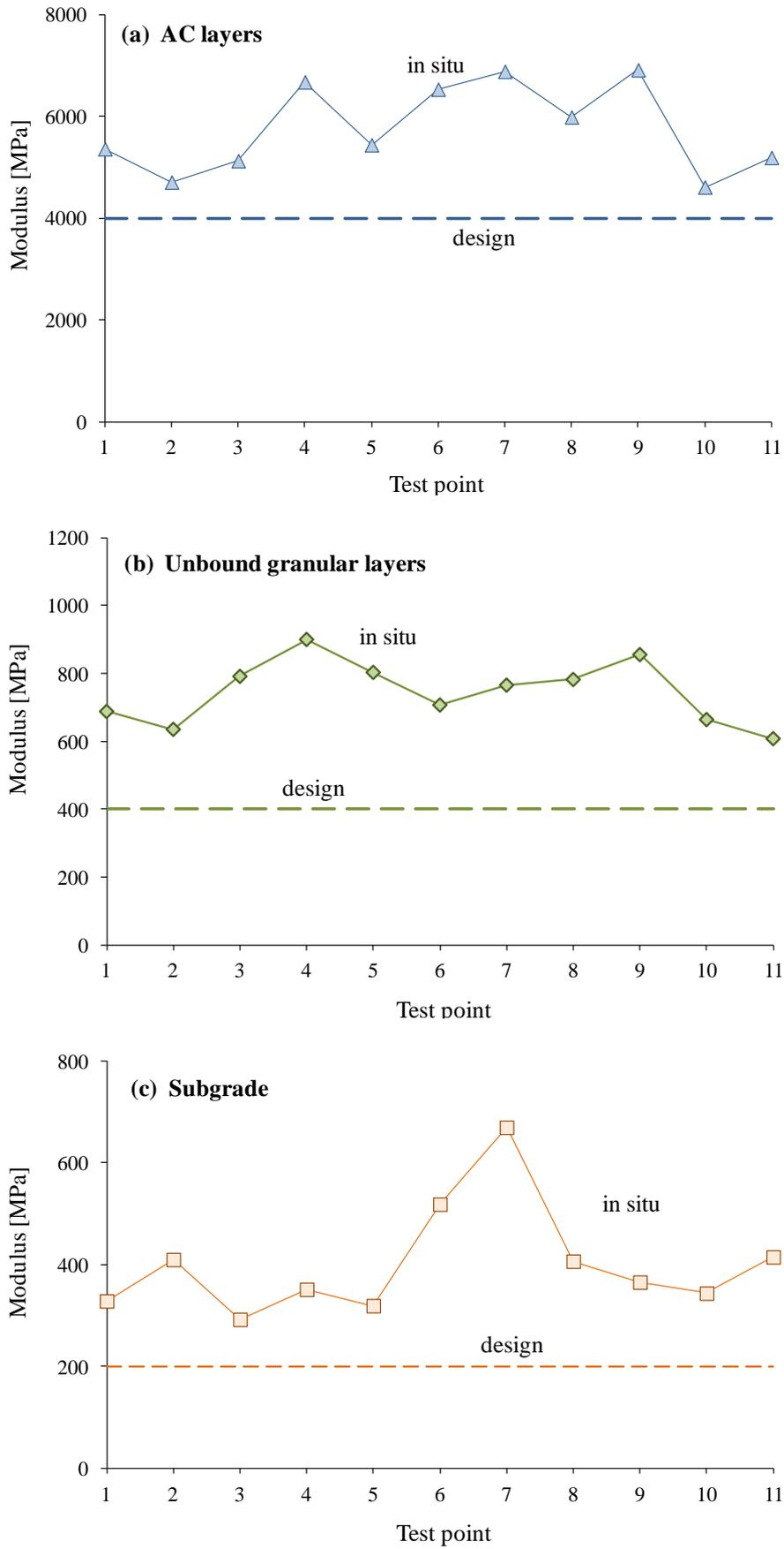
Figure 2: Back-calculated layer moduli.
