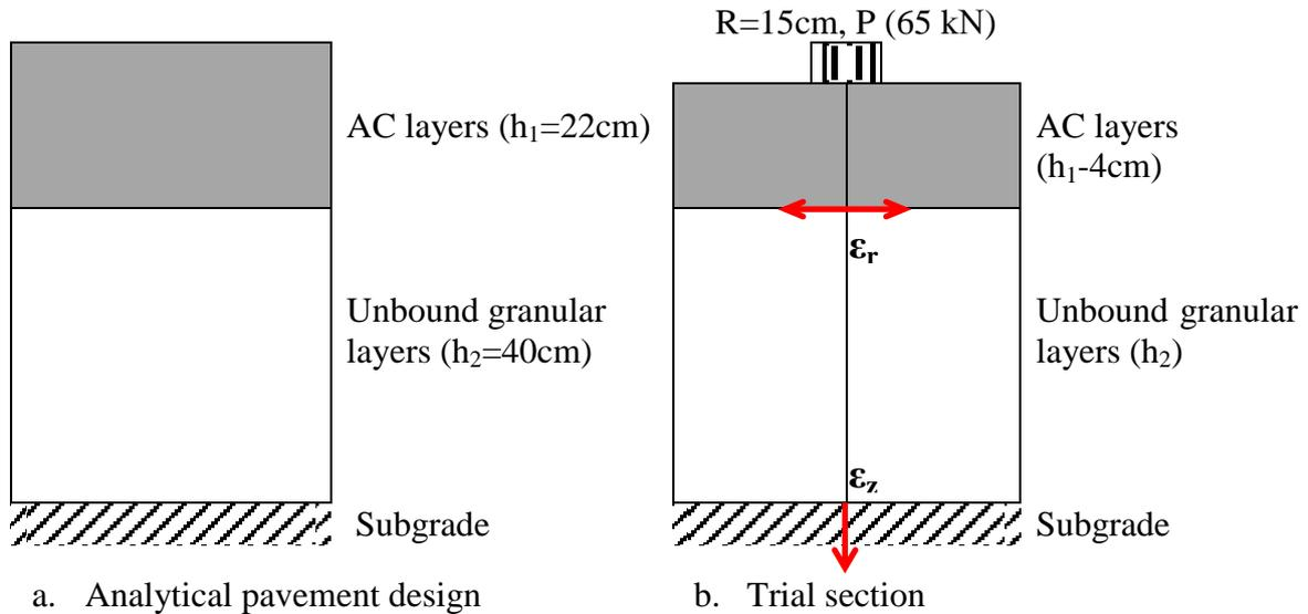
Figure 1: Pavement modeling (cross-section).
