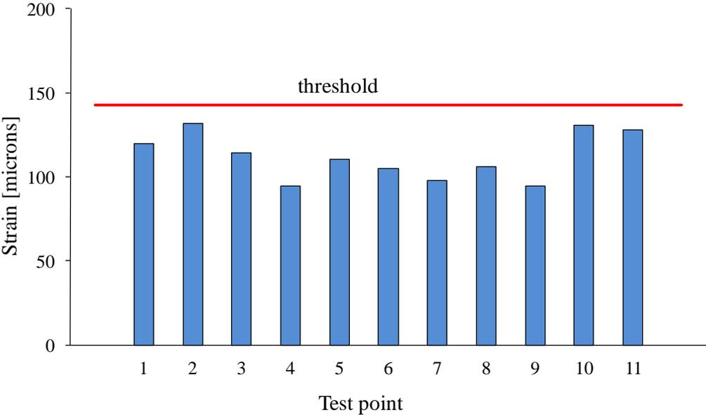
Figure 3: Horizontal (tensile) strains at the bottom of AC layers ( $\epsilon_r$ ).
