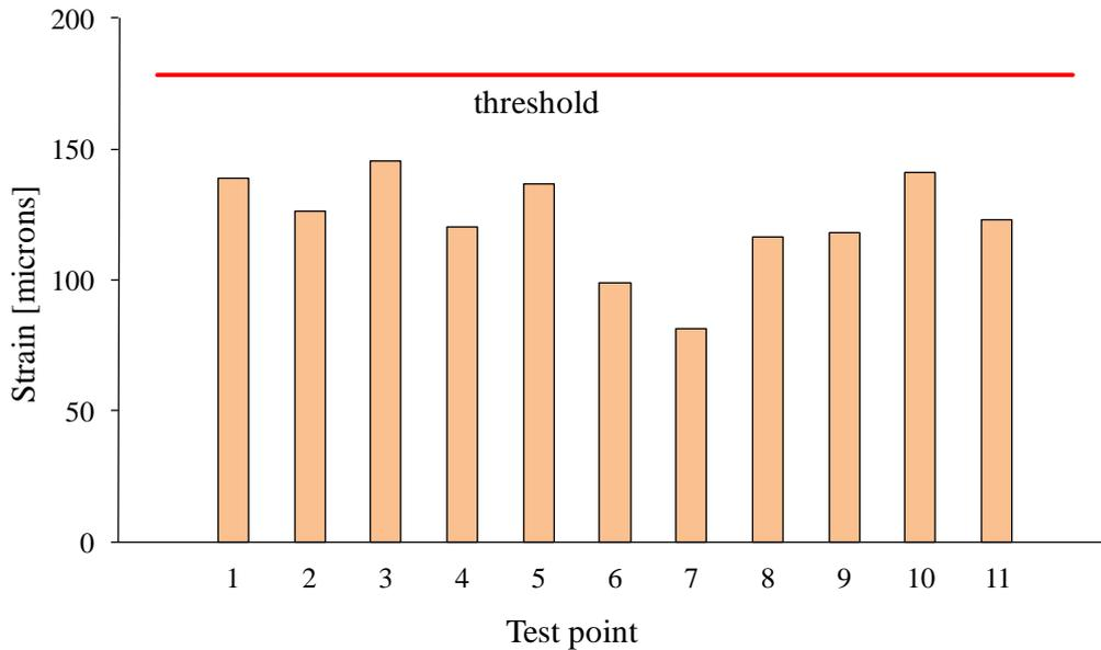
Figure 4: Vertical compressive strains at the top of the subgrade ( $\epsilon_z$ ).
