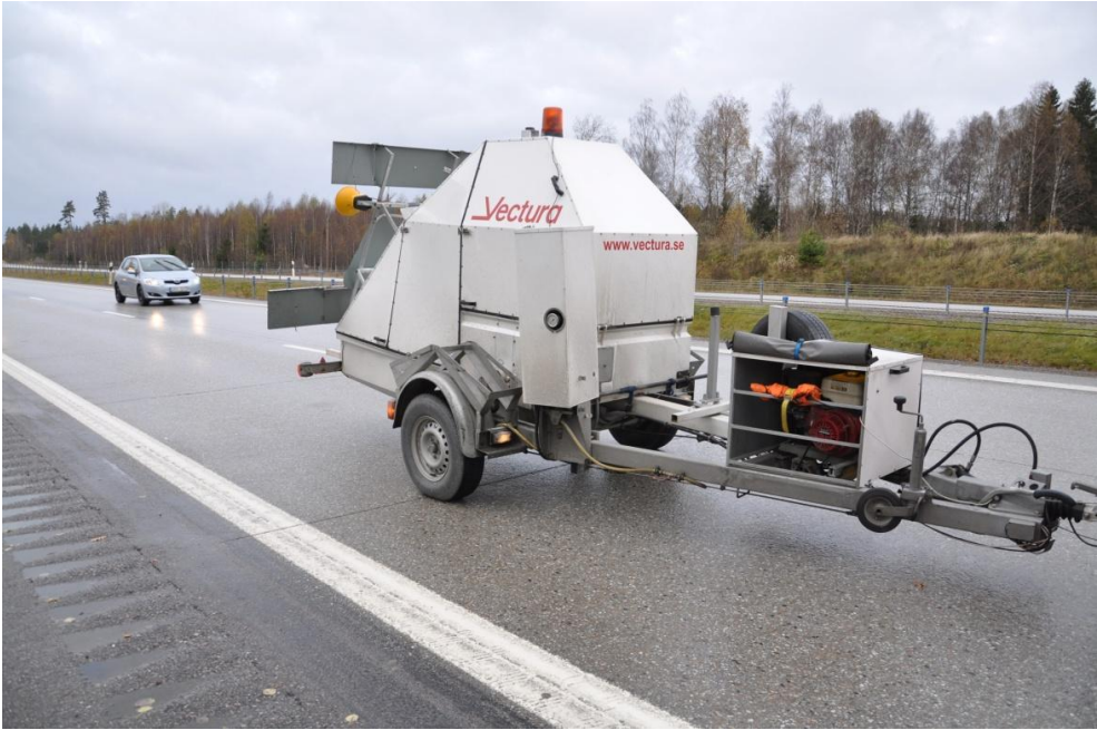
Figure 4: The FWD at E20 testing near the edge of the slab.
