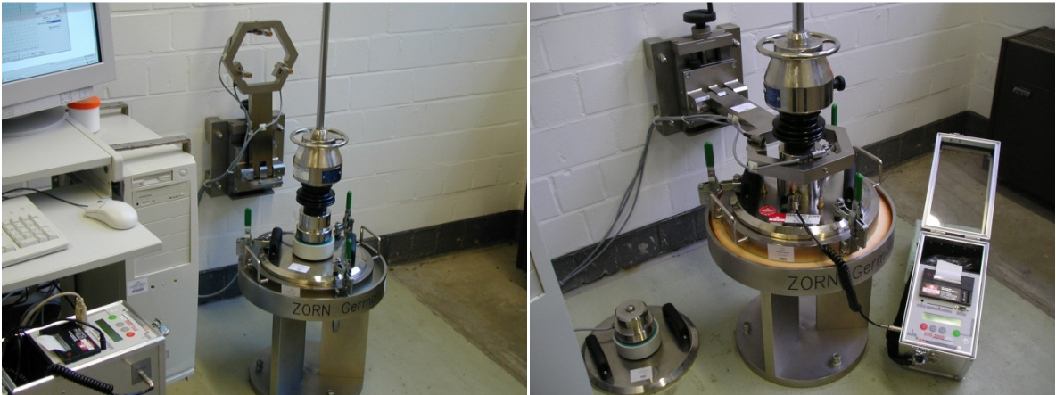
Figure 5: Photos of calibration stand setup for load gear calibration (left) and calibration of the settlement sensor (right)
