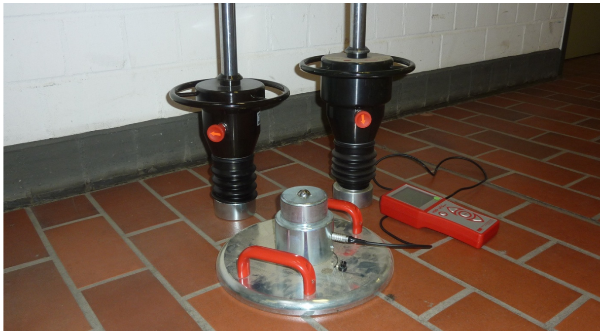
Figure 3: LFWD (left) and MFWD (right) load gear, loading plate and data processing unit
