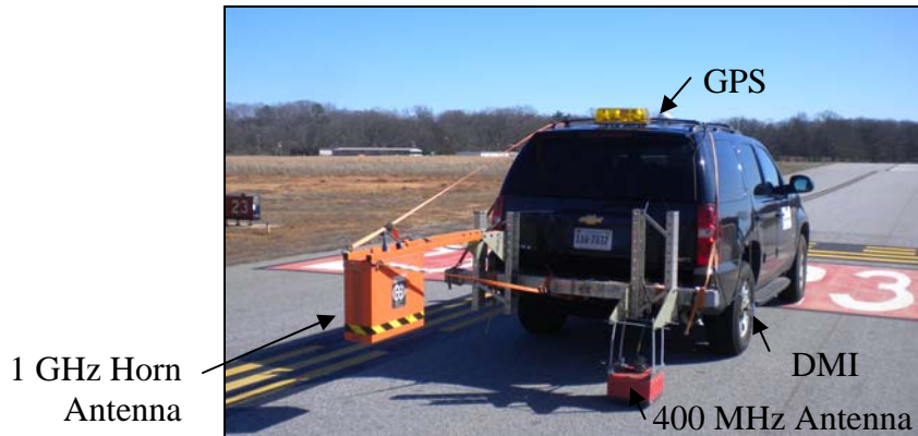
Figure 1: GPR Equipment Setup
