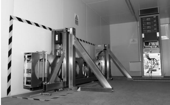
Figure 5a: Measurement beam before fans fitted.
