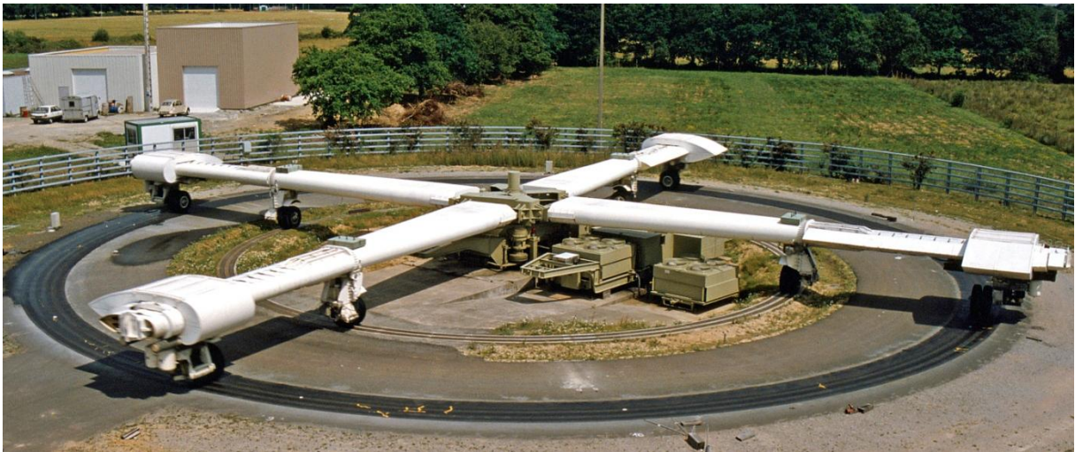
Figure 1. The pavement fatigue carousel of IFSTTAR
