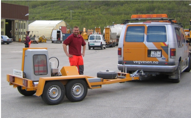
Figure 8: FWD operated by the Norwegian Public Road Administration (NPRA), Region North
