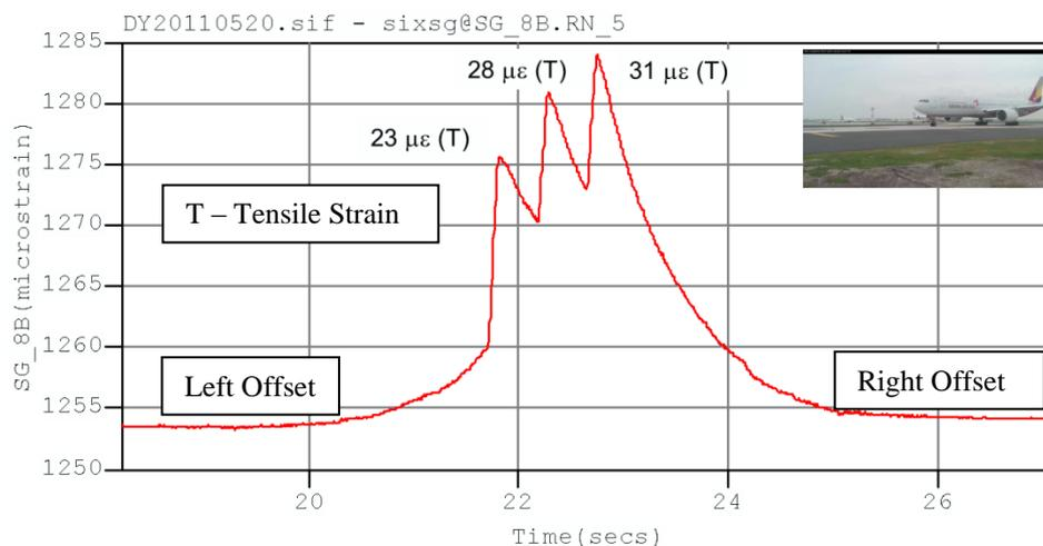
Figure 13: A typical strain gage response located at the bottom of the slab.
