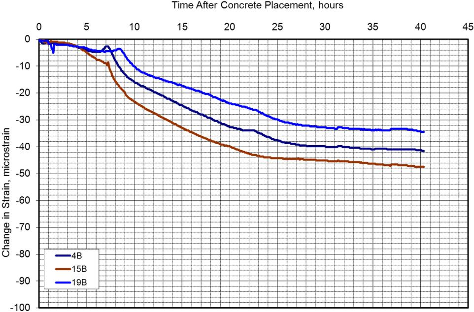
Figure 11: Early age concrete strains at bottom of the slab.
