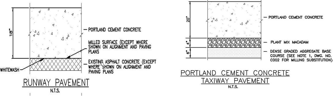
Figure 2: Runway and taxiway pavement cross sections. (1 inch = 2.54 cm)
