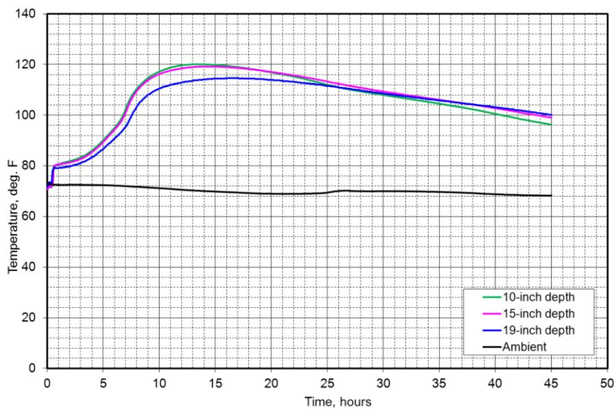
Figure 10: Temperature data collected during initial age of concrete (1 inch = 2.54 cm).
