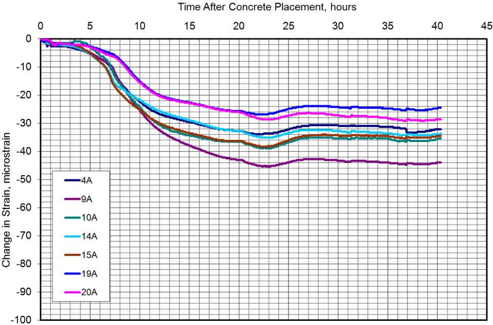
Figure 12: Early age concrete strains at mid-depth of the slab.
