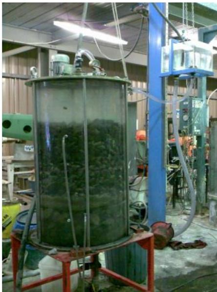
Figure 2: Large scale permeability apparatus
