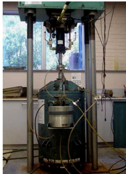
Figure 3: Large scale triaxial apparatus
