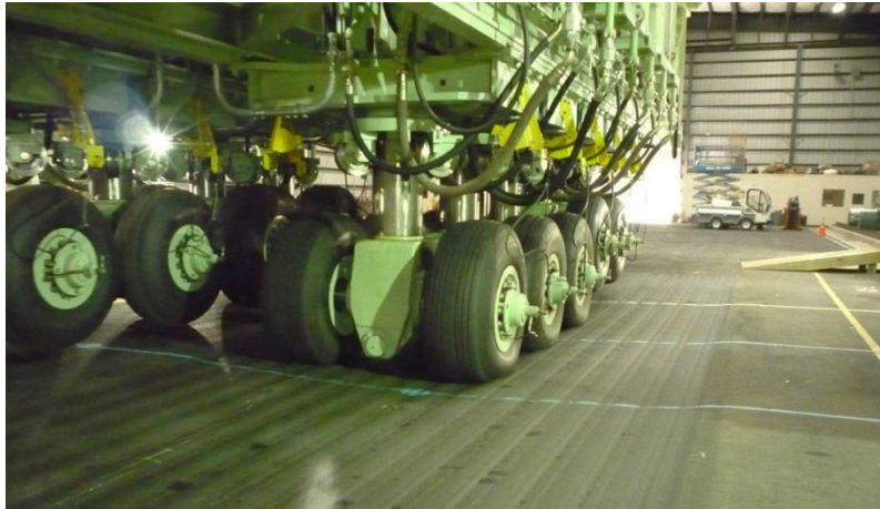
Figure 4: Trafficking the ten-wheel group of wheels on CC5 at 31.8 MT (70,000 lb).
