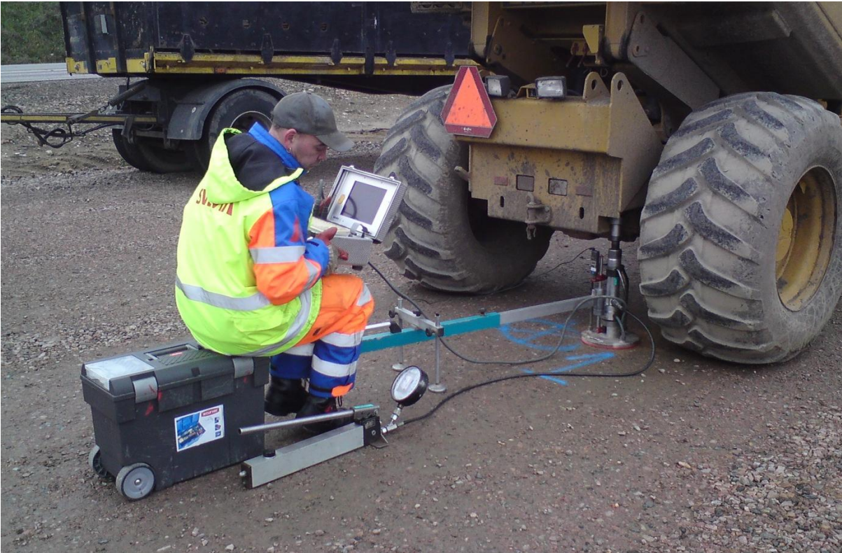
Figure 1: Plate Load Test equipment with jack and data collection unit.
