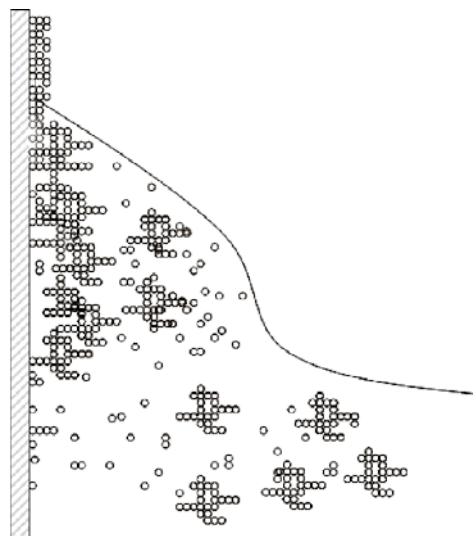
Figure 1: Illustration of thin film formation by dip-coating from a sol of nanoparticles.
