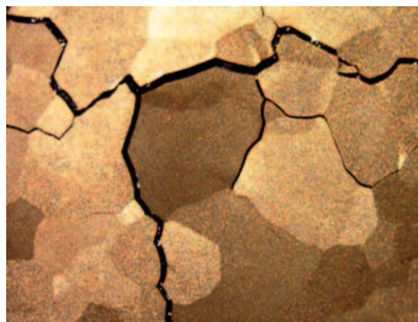
Brittle grain boundaries of pure aluminum.
